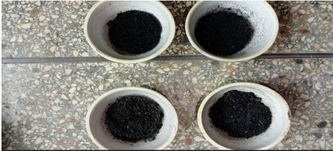
Figure 3.3: Substrates after drying in the muffle furnace at 900 °C
