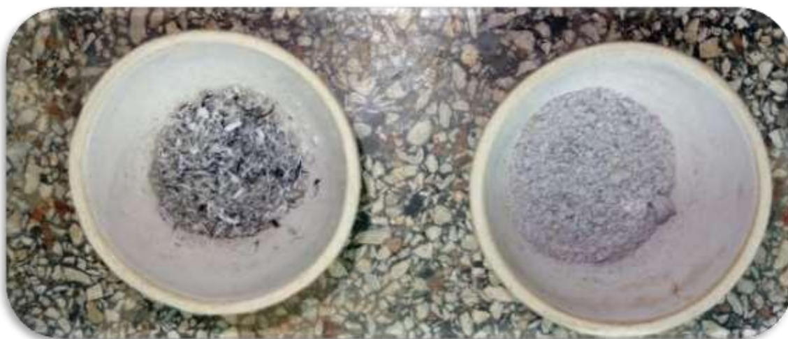
Figure 3.4: Substrates after drying in the muffle furnace at 550 C° of the ash.
