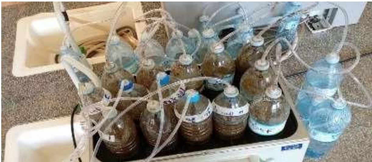
Figure 3.5: Experimental setup of anaerobic co-digestion of CD and MS
