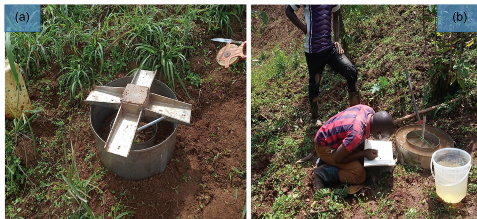
Figure 4. Authors setting up the infiltration experiments in the field (2020).
