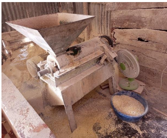
Photo 8: Polishing of HMT-treated maize grains using the traditional maize huller
