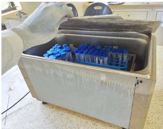
Photo 10: Digestion of maize flour in magnetic stirrer water bath at 37°C for 5 min at 170 rpm
