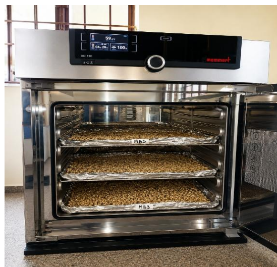
Photo 7: Maize grain drying after application of HMT to reduce the moisture content to 10-11%
