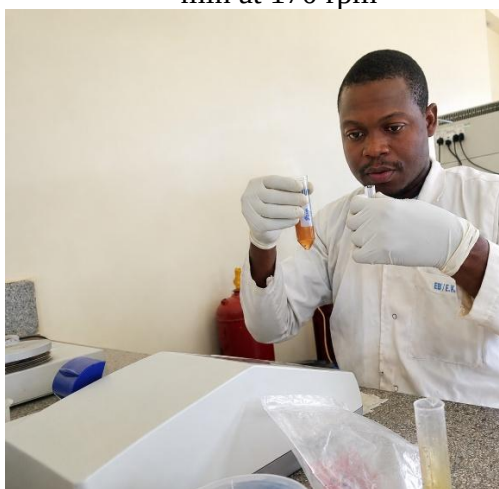
Photo 12: Spectrophotometric Reading of Color Intensity Used to Calculate Released Glucose (Corrected vs. Blank)
