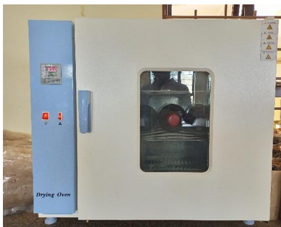
Photo 6: Maize grains packed in glass bottles and heated using an electric hot-air drying oven (Heat application of HMT)
