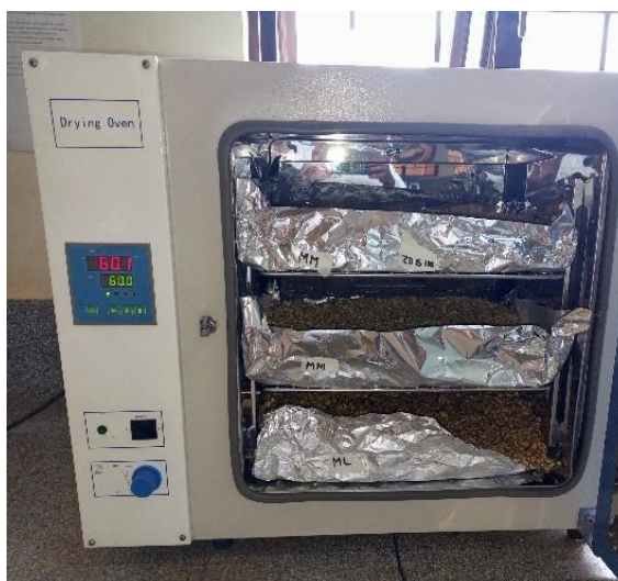
Photo 7: Maize grain drying after application of HMT to reduce the moisture content to 10-11%
