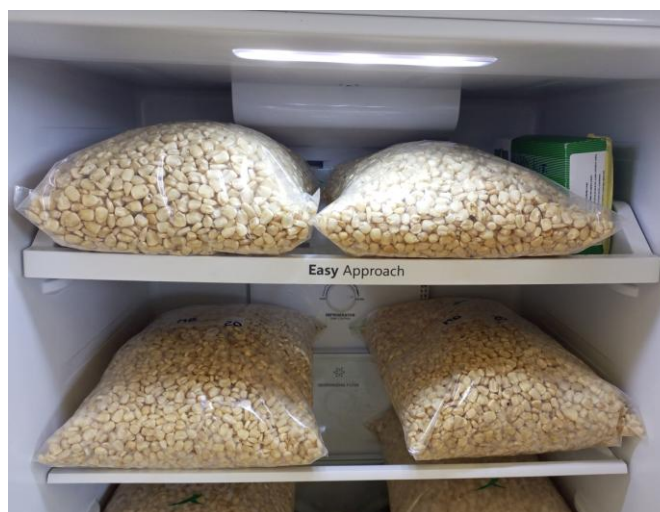
Photo 4: Maize grains Sealed in Polyethylene Zipper Bags after adjusting moisture content, keep in Fridge at 4°C for 24 hours for moisture equilibration
