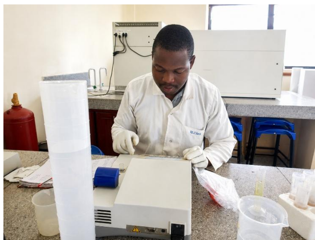
Photo 12: Spectrophotometric Reading of Color Intensity Used to Calculate Released Glucose (Corrected vs. Blank)
