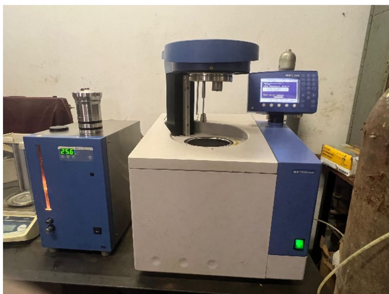
Figure 2. The bomb calorimeter (Model: C2000 basic, IKA Co., Germany) used to determine the higher heating value of the banana plant wastes.
